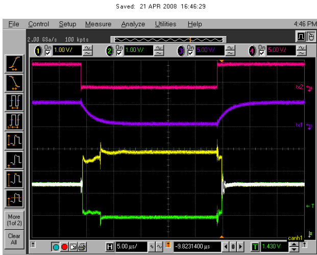
Figure 9. Signal repetition in case different nodes coincidentally transmit on both branches. Blue – TxD signal of the node on bus1 (delayed with an RC constant); magenta – TxD signal of the node on bus 2; yellow and green – bus voltage on bus1.
